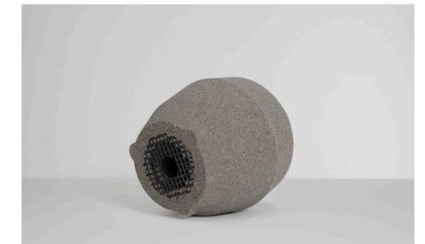
Specifically designed for use in hand moulding. The elimination of the traditional breaker ensures optimised, and reliable feeding of the casting due to the increased contact of the riser at the casting. Easy riser removal is ensured due to the addition of the refractory mesh and the predetermined fracture point within the riser neck.
