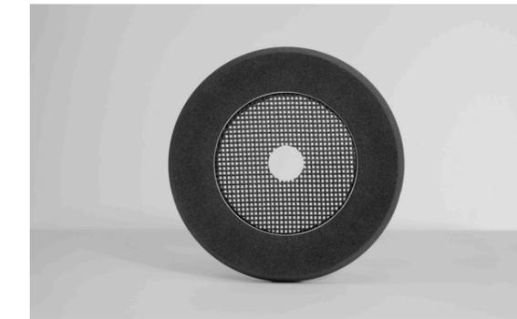
Breaker core technology which can be applied with highly exothermic -Thermo Risers, cylindrical or cylindrical reduced EXO-ISO fiber sleeves, consisting of a high temperature resistant ceramic media to prevent sintering, in combination with a refractory mesh placed directly at the casting surface ensures the formation of a clean predetermined breaking point along the entire riser neck cross-section.
